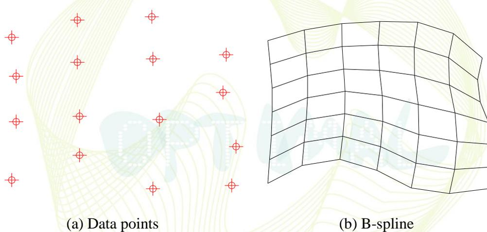
**Figure 6. B-spline surface.**
