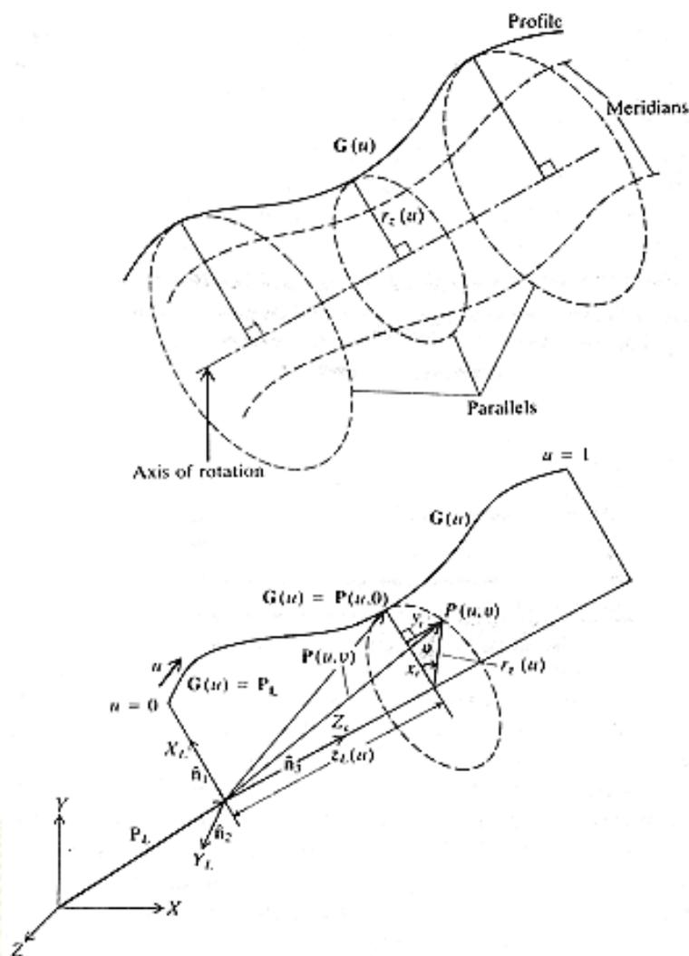
Figure 11. Parametric representation of a surface of revolution.
